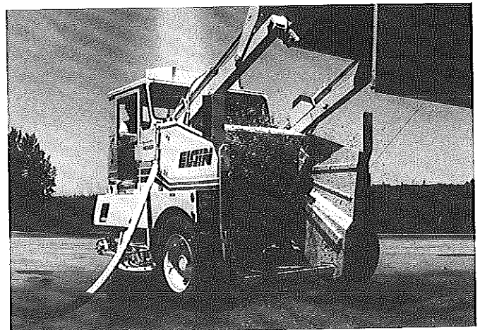
CONVEYOR FLUSHING (Shown with hopper raised)
